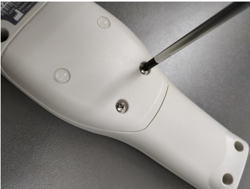
Figure 18 Remove only two screws from battery casing
